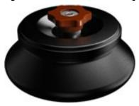
The CF 12×5-24R is a fixed-angle rotor designed to centrifuge up to twelve 5 mL tubes at a 45° angle to the axis of rotation. Applications for this rotor include general pelleting of bacteria, subcellular organelles, viruses, mitochondria, chloroplasts, and algae. Up to 60 mL of sample volume can be centrifuged per run.
