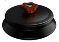
The CF  $36\times0.5$ -24R is a fixed-angle rotor designed to centrifuge up to thirty-six 0.5 mL tubes at a  $45^\circ$  angle to the axis of rotation. Applications for this rotor include general pelleting of bacteria, subcellular organelles, viruses, mitochondria, chloroplasts, and algae. Up to 18 mL of sample volume can be centrifuged per run.
