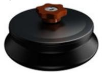
The CF  $24 \times 2-24R$  is a fixed-angle rotor designed to centrifuge up to twenty-four 2 mL tubes at a  $45^{\circ}$  angle to the axis of rotation. Applications for this rotor include general pelleting of bacteria, subcellular organelles, viruses, mitochondria, chloroplasts, and algae. Up to 48 mL of sample volume can be centrifuged per run.
