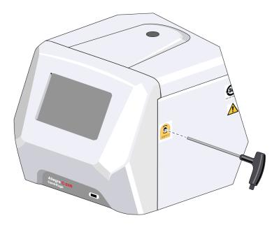
Open the door cover by turning the 5 mm T-handle Allen wrench counterclockwise with half a circle.
