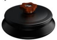
The CF  $32\times0.2$ -PCR-24R is a fixed-angle rotor designed to centrifuge up to thirty-two 0.2 mL tubes at a  $45^\circ$  angle to the axis of rotation. Applications for this rotor include accommodating and processing small volume samples, typically in 0.2 mL microcentrifuge tubes or PCR tubes or strips. Up to 6.4 mL of sample volume can be centrifuged per run.
