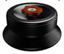
The CF  $18\times2-24R$  is a fixed-angle rotor designed to centrifuge up to eighteen 1.5/2 mL tubes or 2 mL spin column at a  $45^{\circ}$  angle to the axis of rotation. Applications for this rotor include DNA and RNA extraction. Up to 36 mL of sample volume can be centrifuged per run.
