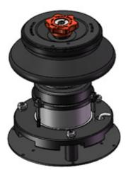
2 Insert a 5 mm T-handle Allen wrench into the centered circle hole of the rotor cover, and tighten the Allen screw in a clockwise direction (about 5 rotations).
