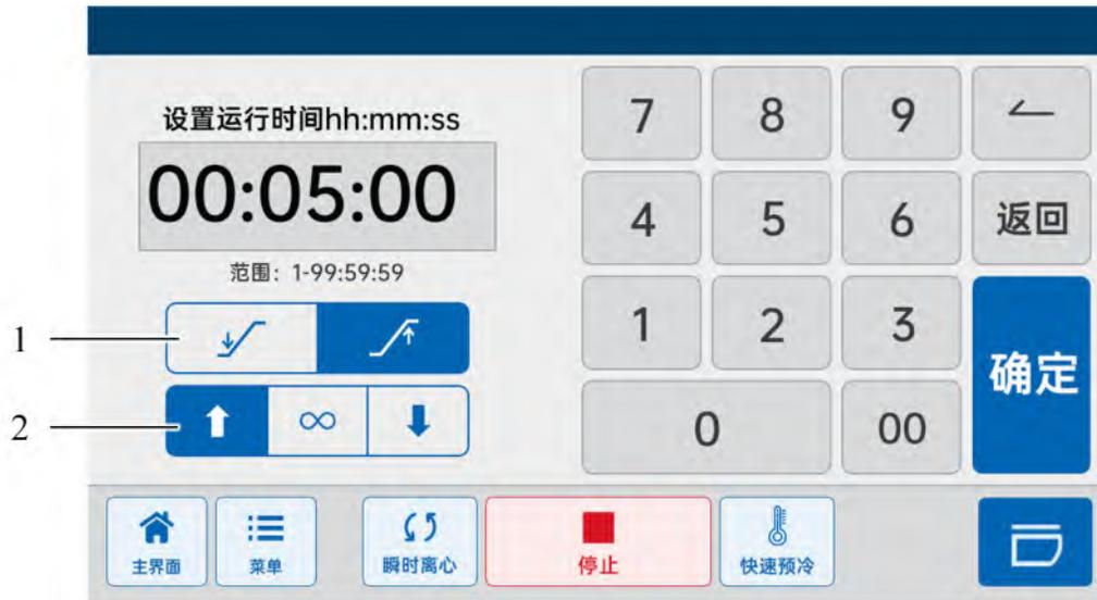
1. 达速计时/启动计时：可切换计时方式为到达设定转速开始计时或启动运行同步计时。
